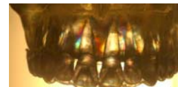
Figure 9. THIN ALIGNER 0.25mm Above is the photoelastic model with the thin aligner inserted. Notice that the stress distribution in both number of fringes and proximity of fringes are less around the centrals and laterals, area of tooth movement.
