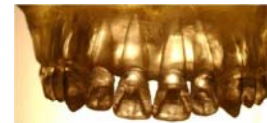
Figure 6. Above is the photoelastic model with no aligner. Notice that there are no stress associated with any of the teeth and the model is stress free prior to testing. Stress is visualized as areas demonstrated by rainbow like banners with different colors reflective of various intensity. The closer the fringes are to one another the higher the concentration of stress and the greater the number of fringes denotes greater intensity of stress.
