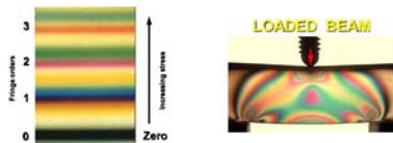
Figures 1 and 2: Schematic representation of stress on a photoelastic model with load. The color layers are referred to as fringes. Notice that there are greater number and greater proximity of fringes decrease as you go further from the load.
