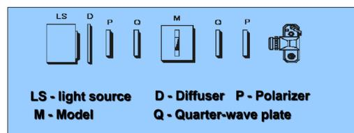
Figure 2. SCHEMATIC REPRESENTATION OF THE PHOTOELASTIC SET-UP
