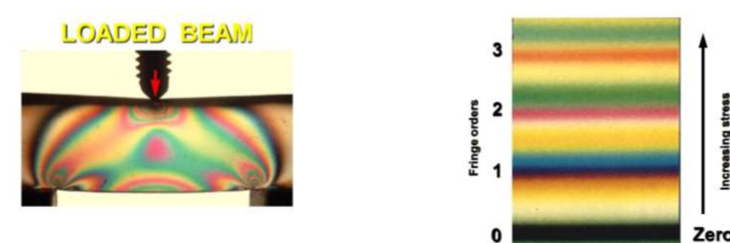
Figure 1. PHOTOELASTIC INTERPRETATION Above represents load exerted on a photoelastic model. Note the increased stress in the proximity of the load-model interface. Number of fringes and proximity of fringes decrease as the distance from direct load increase. To the right is a color scale to determine intensity of stress by colors.
