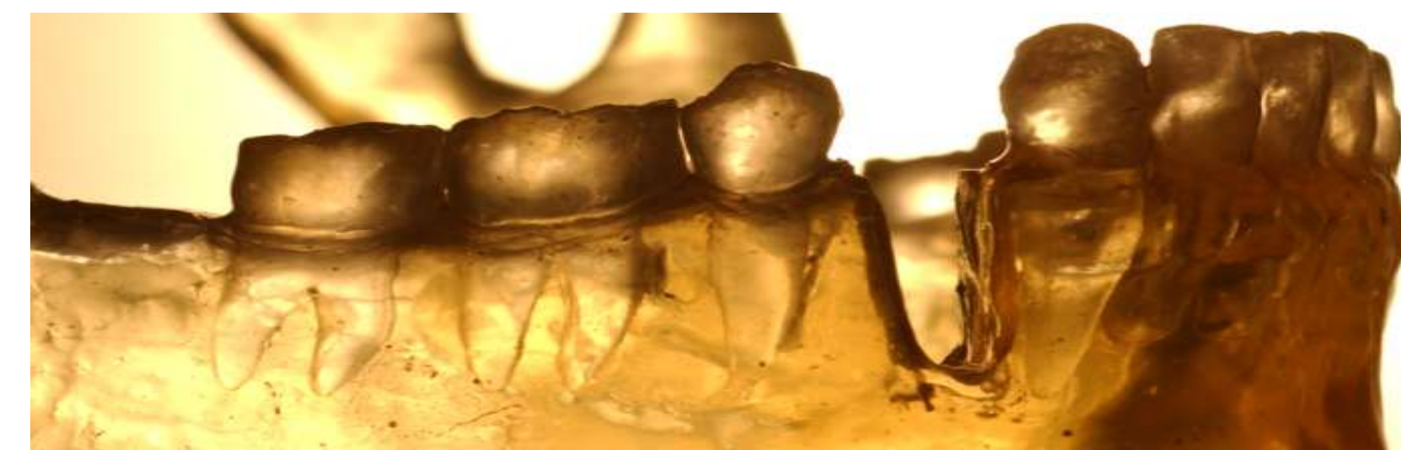
Figure 5. NO APPLIANCE INSERTED ON THE PHOTOELASTIC MODEL Above is the photoelastic model with no orthodontic appliance. Notice that there are no stress associated with any of the teeth and the model is stress free prior to testing. Stress is visualized as areas demonstrated by rainbow like banners with different colors reflective of various intensity. The closer the fringes are to one another the higher the concentration of stress and the greater the number of fringes denotes greater intensity of stress.
