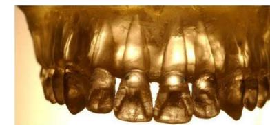
Figure 6. Above is the photoelastic model with no aligner. Notice that there are no stress associated with any of the teeth and the model is stress free prior to testing. Stress is visualized as areas demonstrated by rainbow like banners with different colors reflective of various intensity. The closer the fringes are to one another the higher the concentration of stress and the greater the number of fringes denotes greater intensity of stress.
